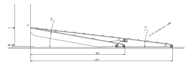
The new extension has a length of 597.2mm and reduces the approach angle from 10 deg to 7.2 deg.
